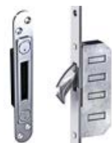
Standard 24mm wide keeps with dust boxes and off-set screw fixing for enhanced security.
