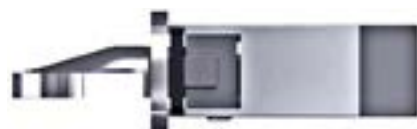
Special design tensile steel handed hook with a 4.5mm chamfer allows a high degree of fitting tolerance for door installation. In addition the hook shape provides low operating forces and helps doors achieve a higher level of weather performance.
