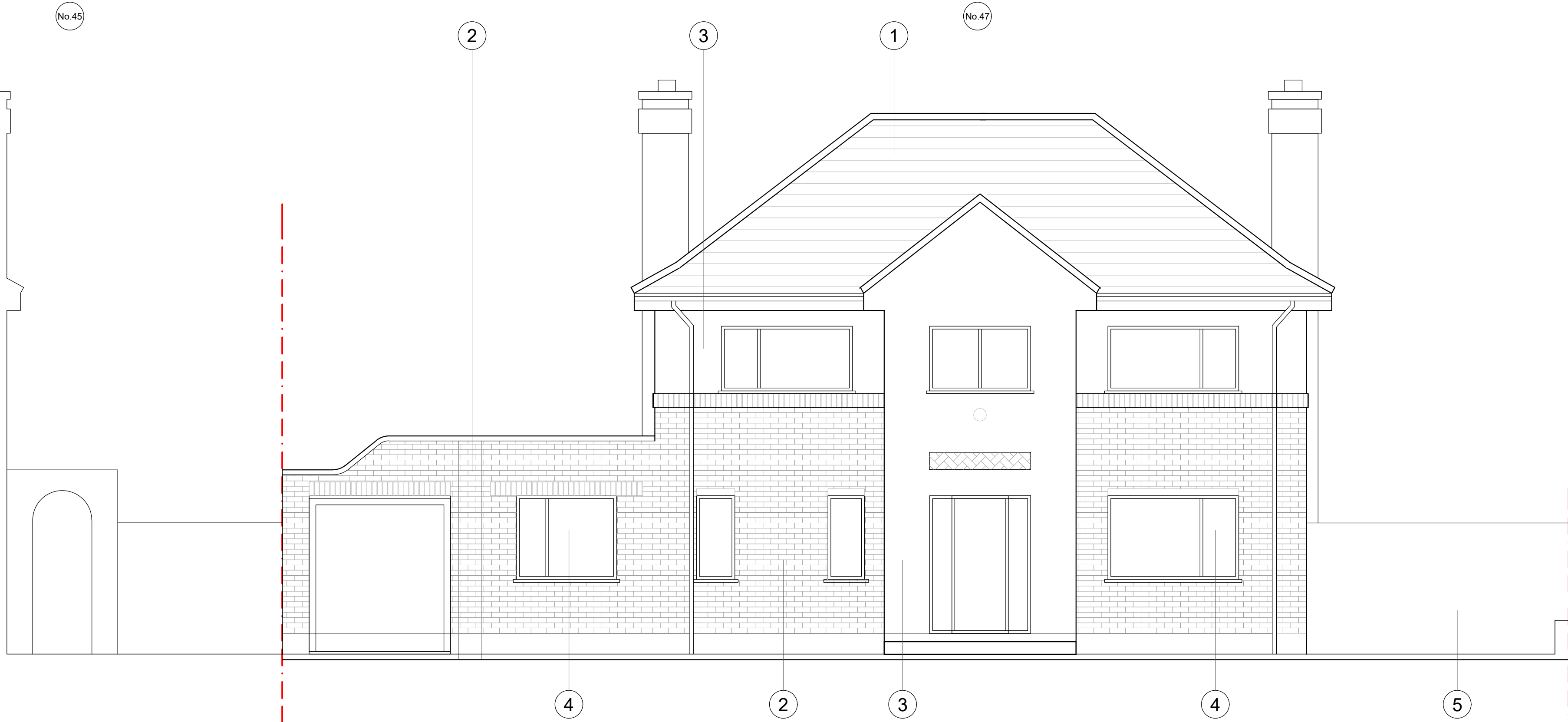
1 EXISTING FRONT ELEVATION 1:50 @ A1, 1:100 @ A3
