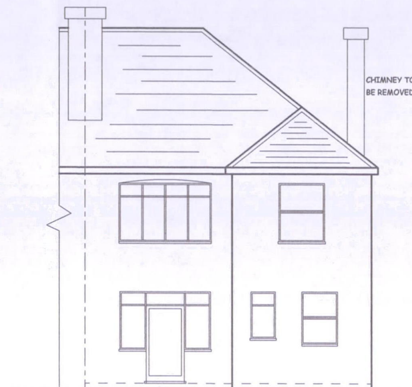
EXISTING REAR ELEVATION
