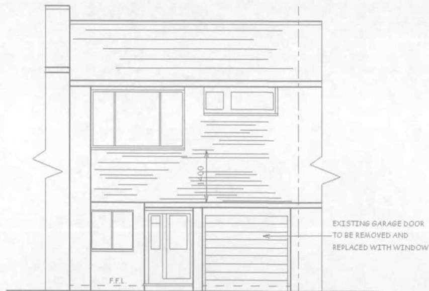
EXISTING FRONT ELEVATION
