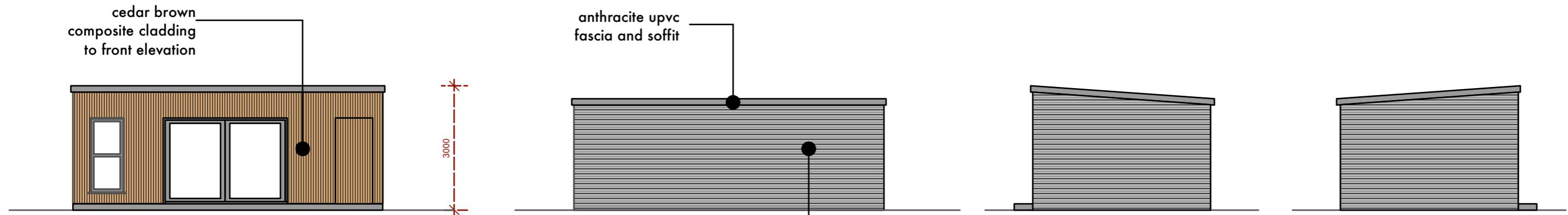
proposed elevations - scale 1:100
