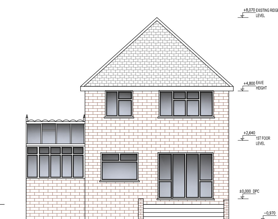
EXISTING REAR ELEVATION 1:100
