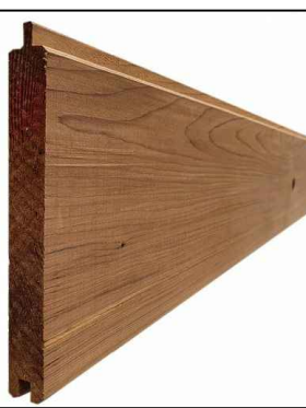
Western Red Cedar No. 2 Clear & Better Tongue & Groove V-Joint vertical timber cladding Board size: 18x94mm, 18x144mm. Grade: No. 2 Clear & Better - 85% Profile: Tongue & Groove connection with a bevelled edge to create a v-shaped shadow line. Surface texture: Smooth.
