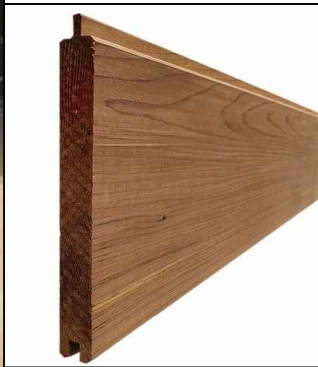
Western Red Cedar No. 2 Clear & Better Tongue & Groove V-Joint vertical timber cladding Board size: 18x94mm, 18x144mm. Grade: No. 2 Clear & Better - 85% Profile: Tongue & Groove connection with a bevelled edge to create a v-shaped shadow line. Surface texture: Smooth.
