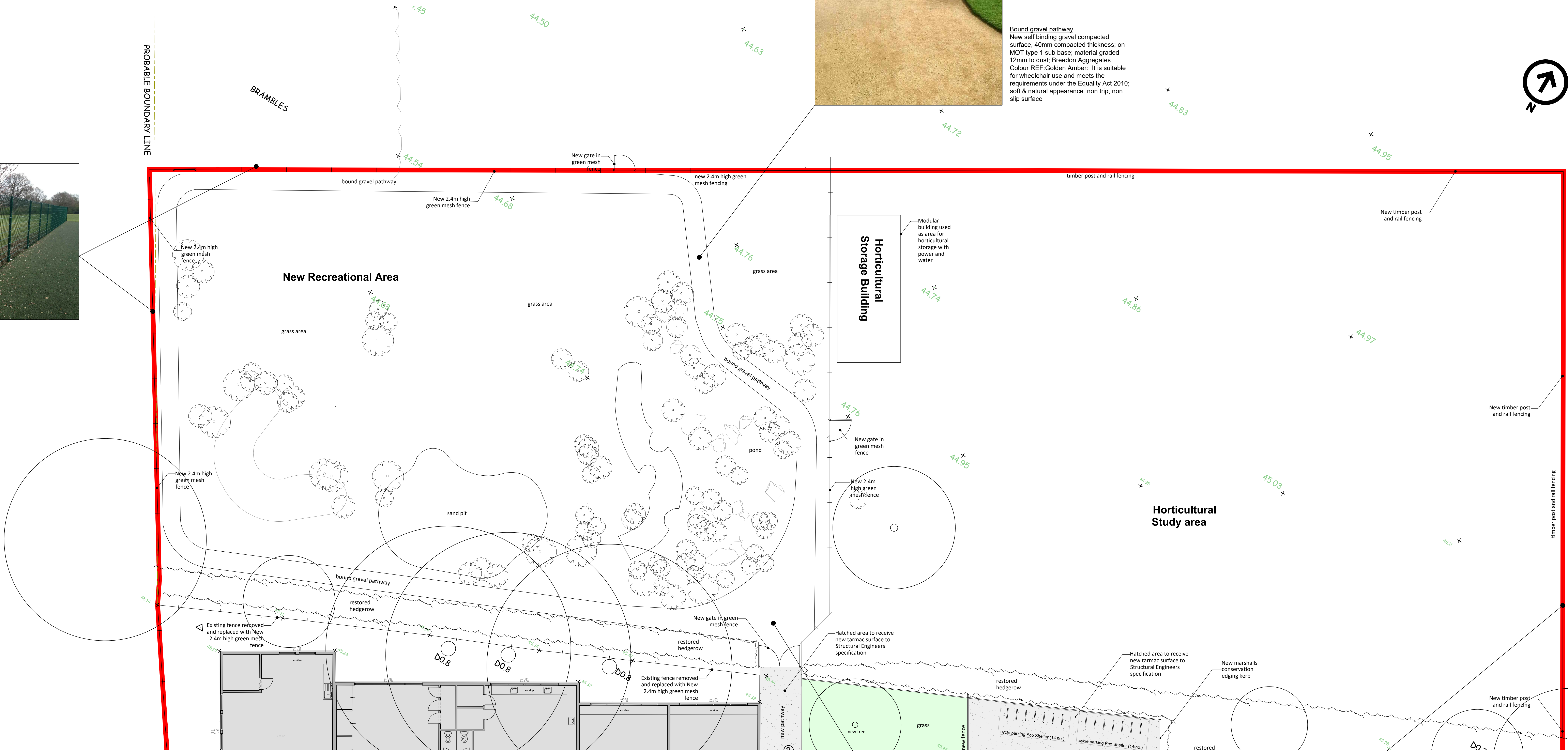
2.4m high green mesh fence Mesh fencing is pre galvanised as well as powder coated RAL 6005 Green
