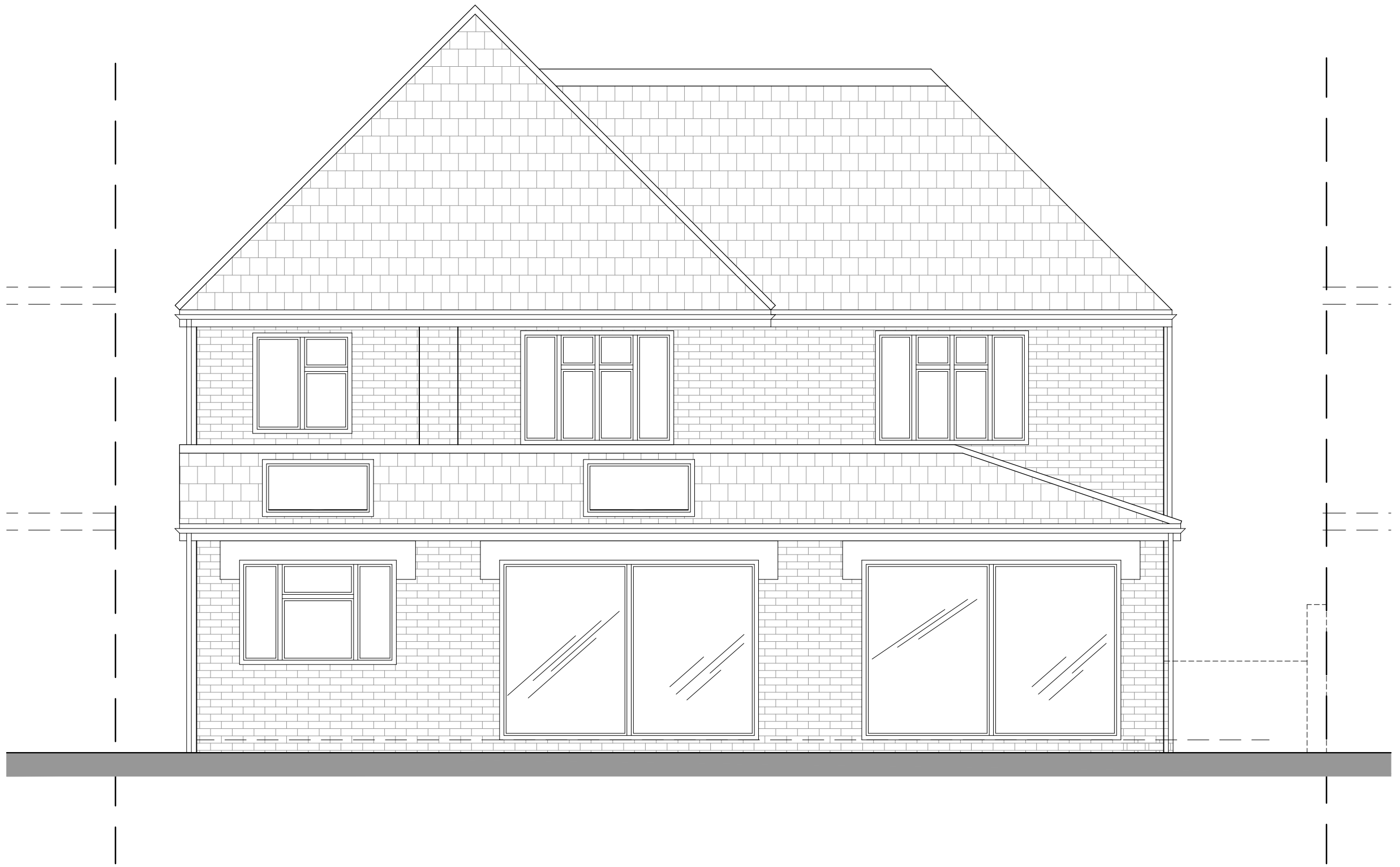
Proposed Rear Elevation Scale 1:50
