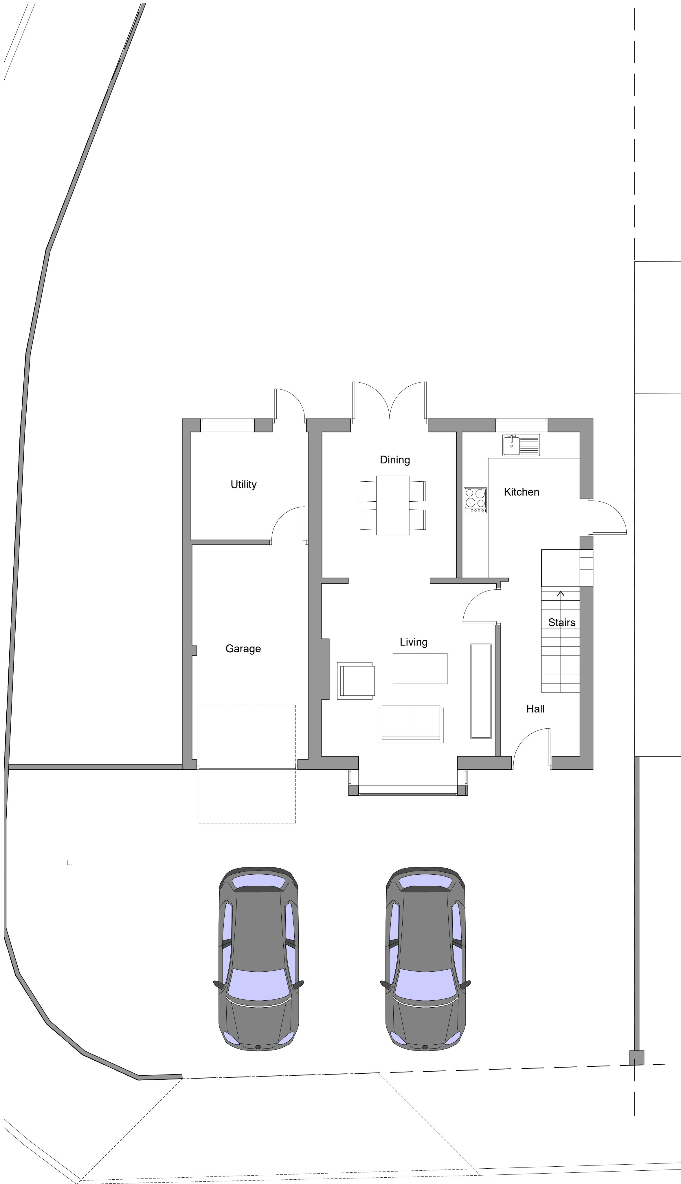
Existing Ground Floor Plan Scale 1:50
