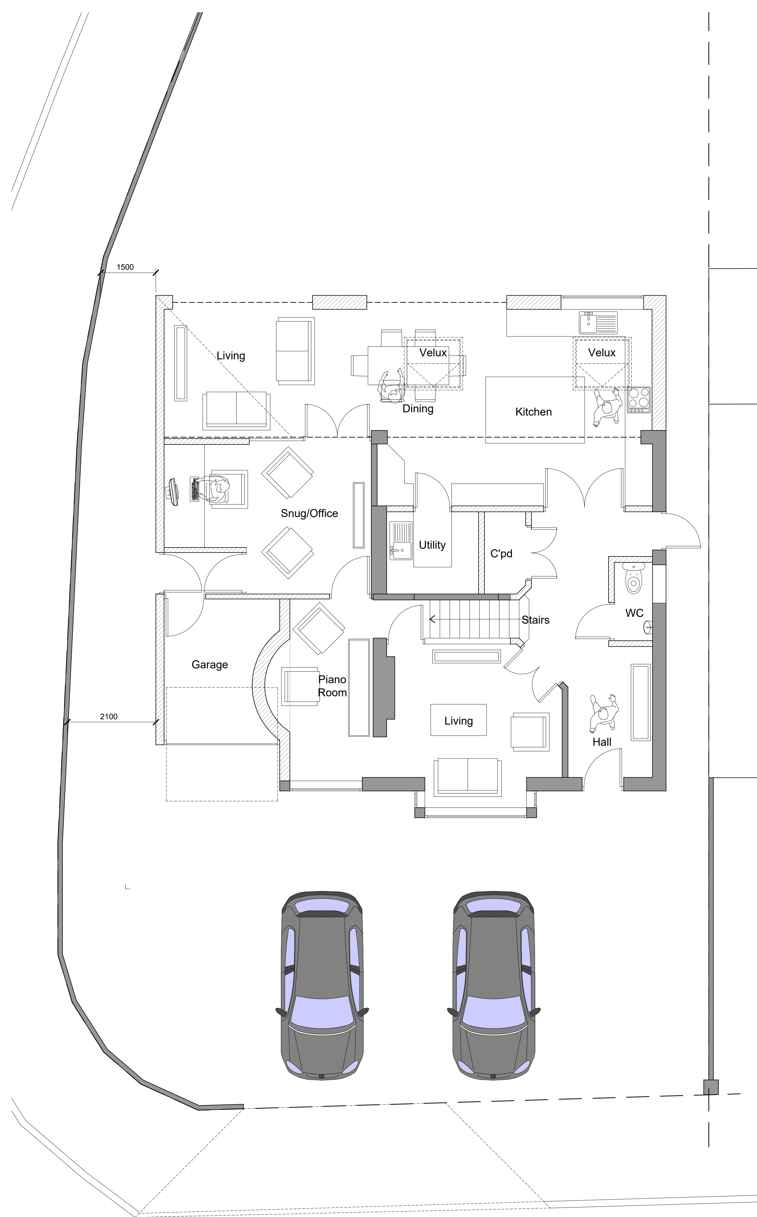
Proposed Ground Floor Plan Scale 1:50
