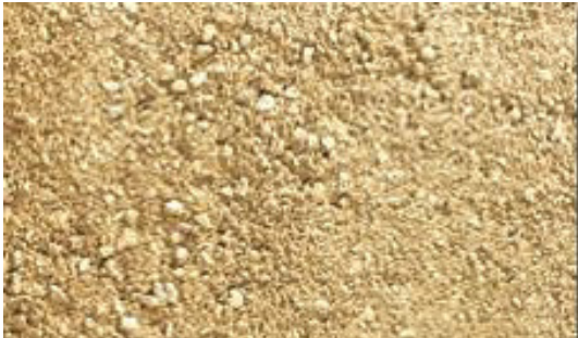
Self-binding gravel for accessible routes.
