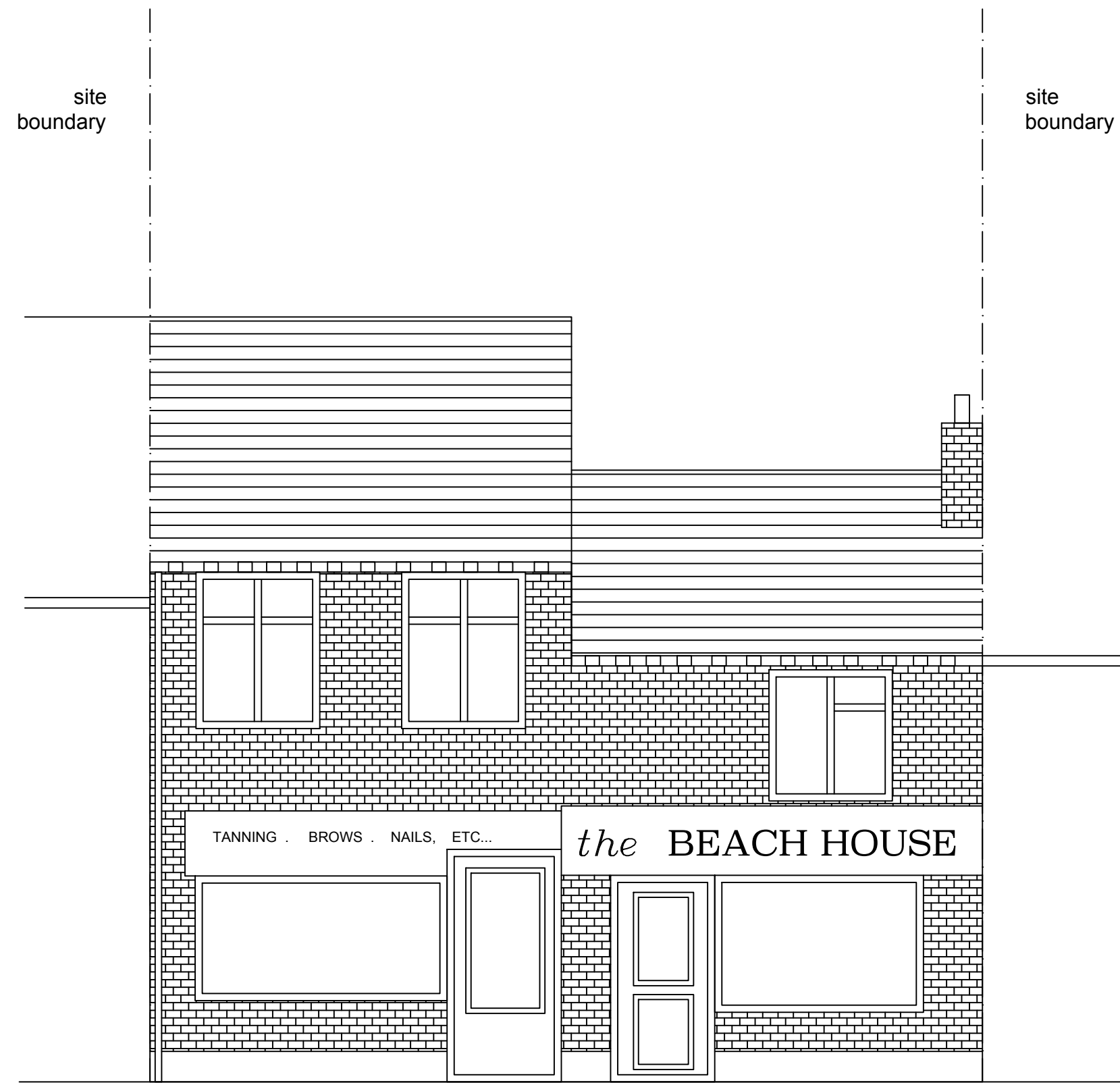
existing front elevation
