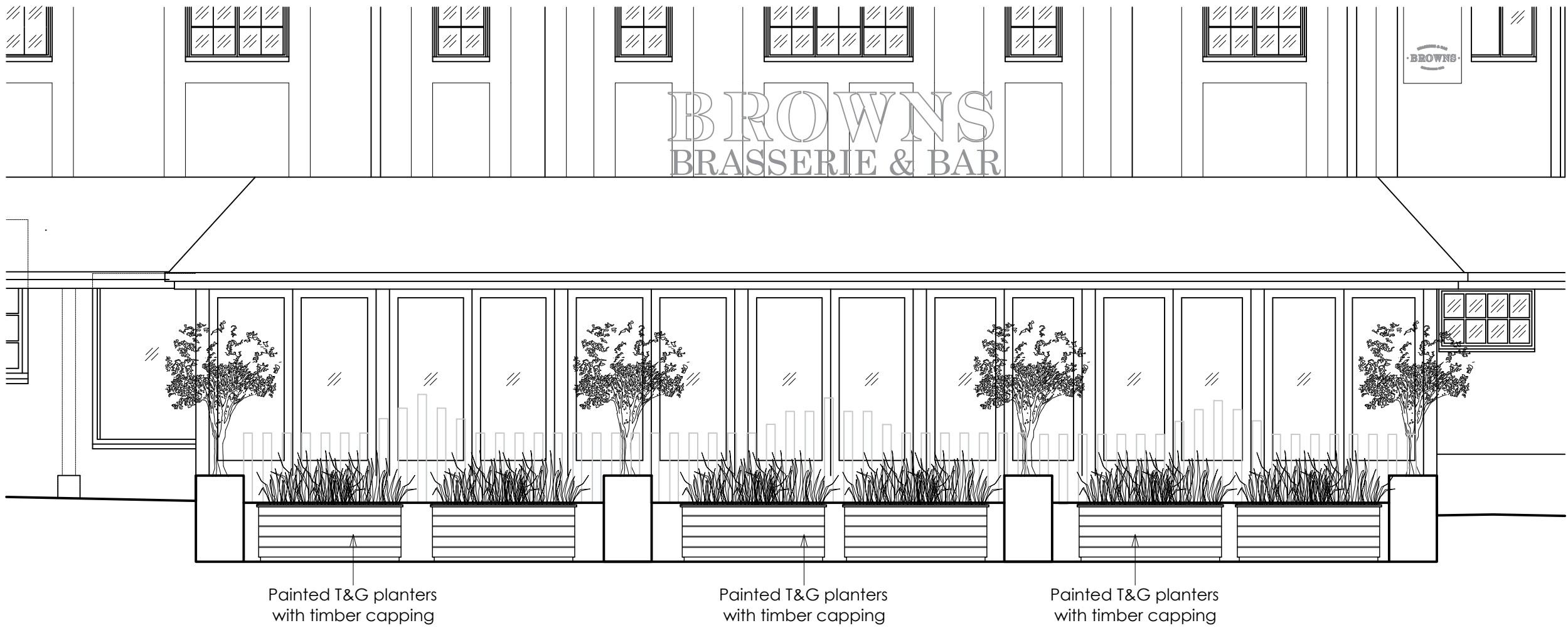
PROPOSED TYPICAL EXTERNAL ELEVATION Scale 1:50
