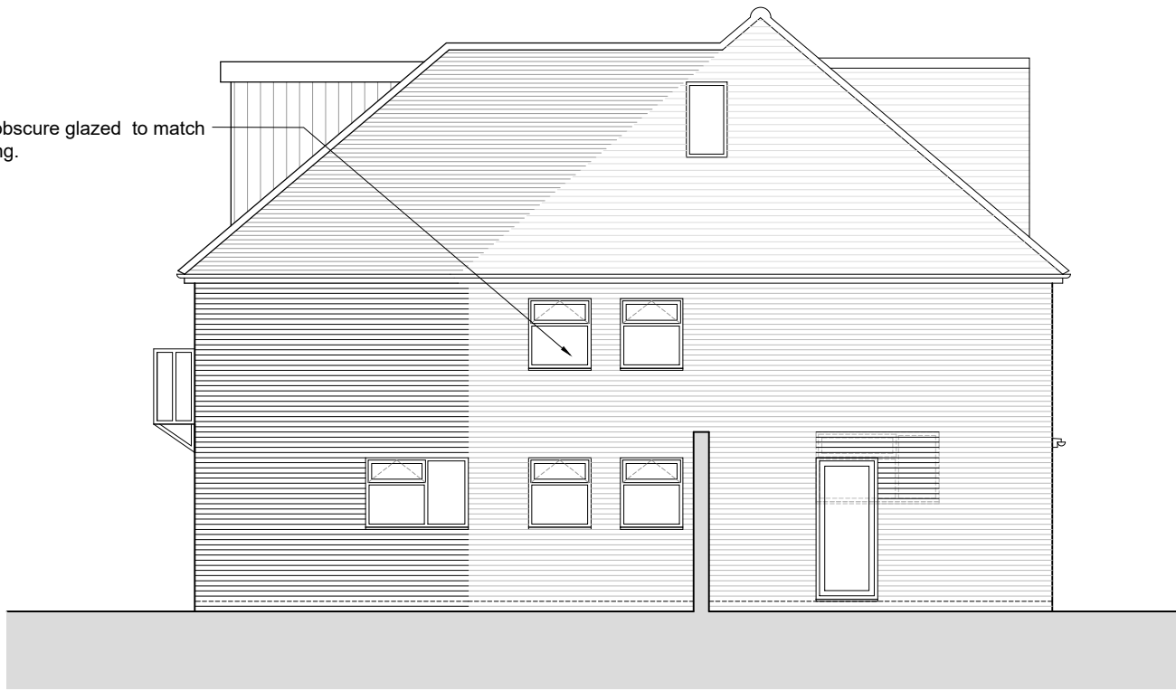
PROPOSED EAST ELEVATION SCALE 1 : 100
