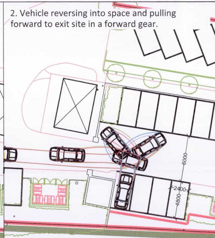
3. Vehicle reversing into space and pulling forward to exit site in a forward gear.
