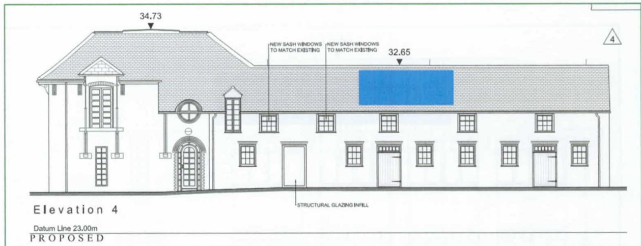
Figure 6 South East Elevation Stables Office Block showing 12 PV Panels
