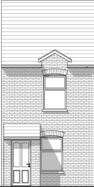
Existing Front Elevation 1:100
