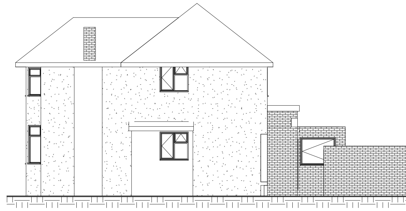
4 Existing Side Elevation 1 : 100
