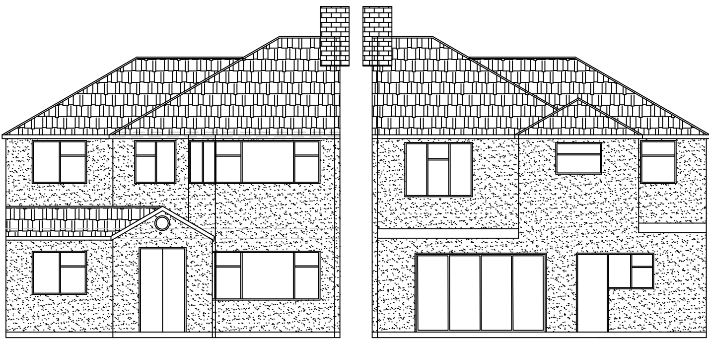
PROPOSED FRONT ELEVATION (Scale 1:100)
