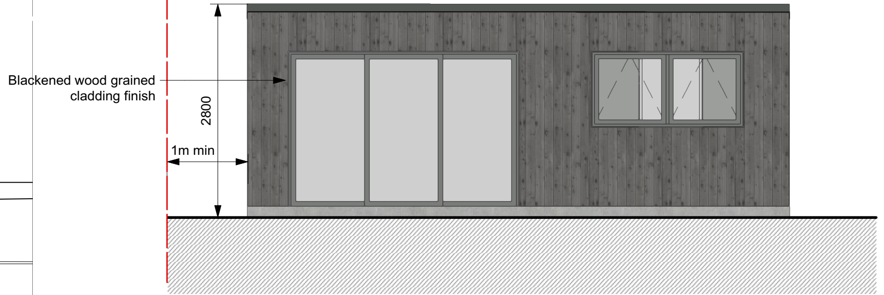
4 Outbuilding - Front Elevation Scale: 1:50
