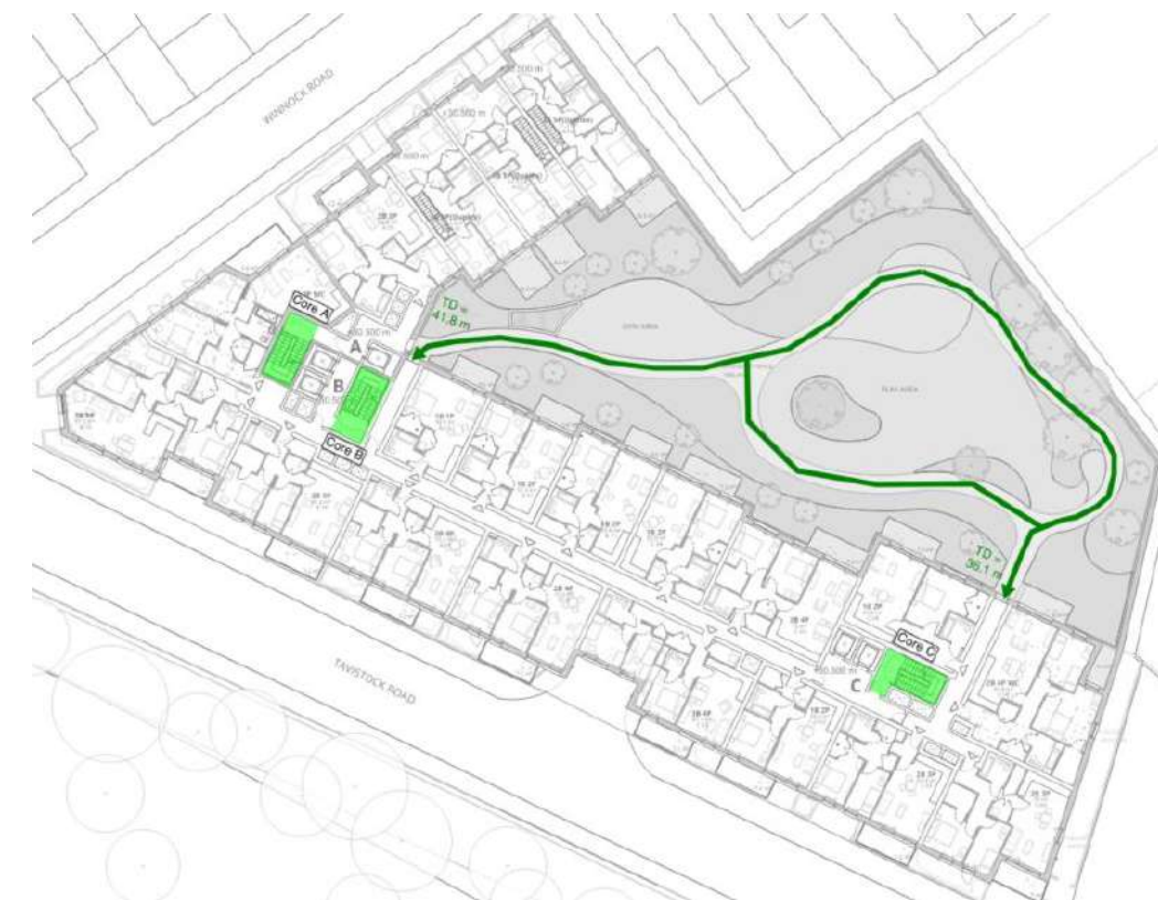
Figure 13 - Podium means of escape
