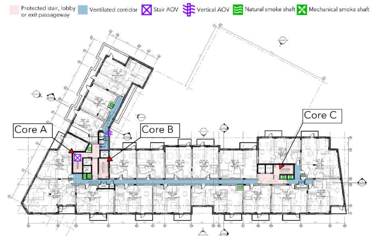
Figure 9 - Proposed common corridor smoke control arrangements Level 02
