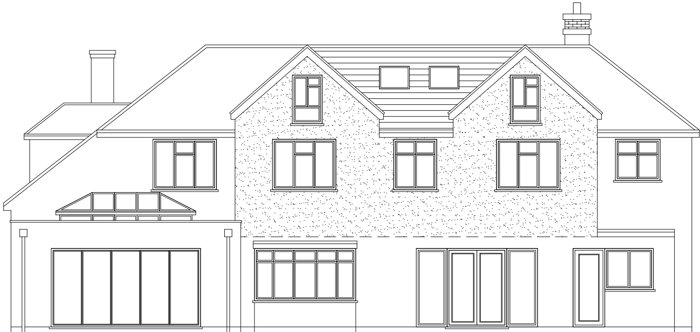
Proposed Rear Elevation Scale 1:100
