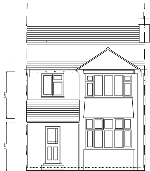
Front Elevation As Existing, Scale 1:100
