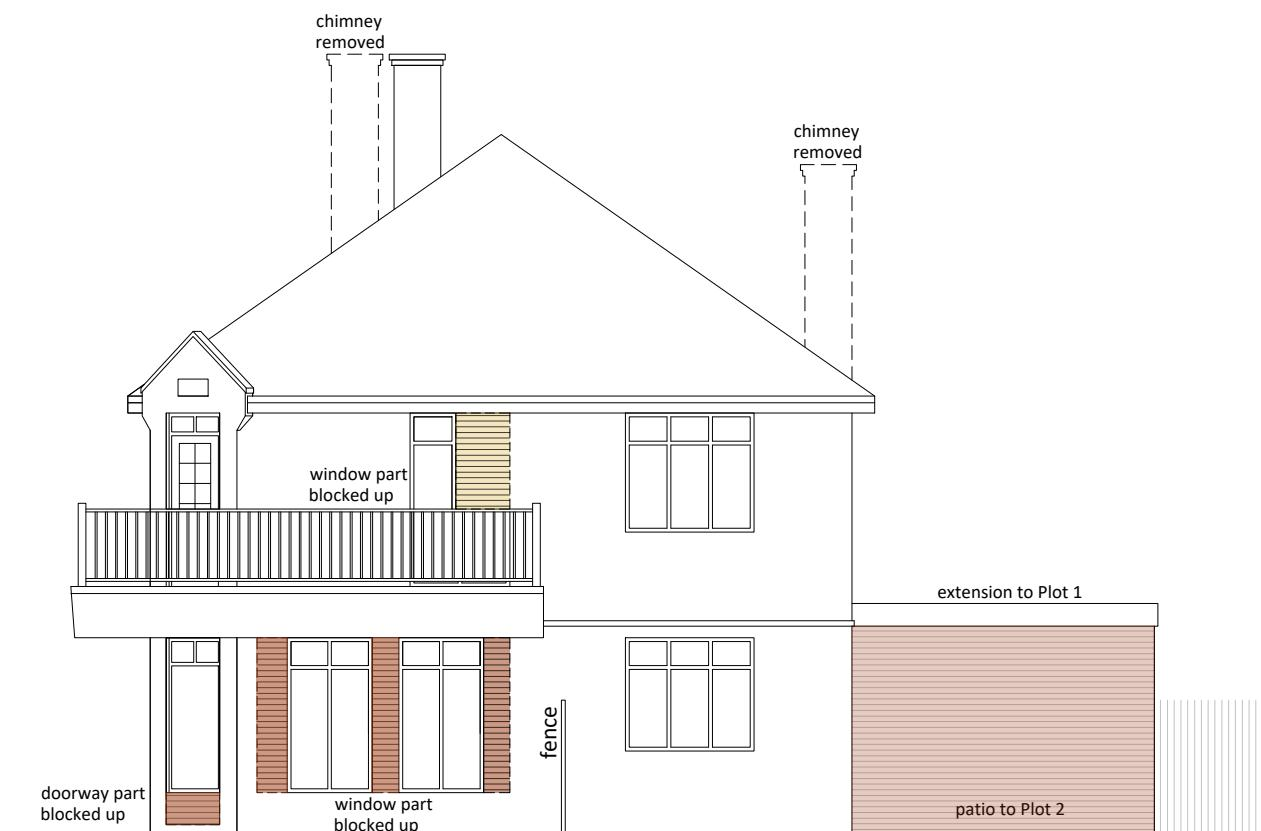
SOUTH-WEST ELEVATION (TO BRAKESPEAR ROAD NORTH)
