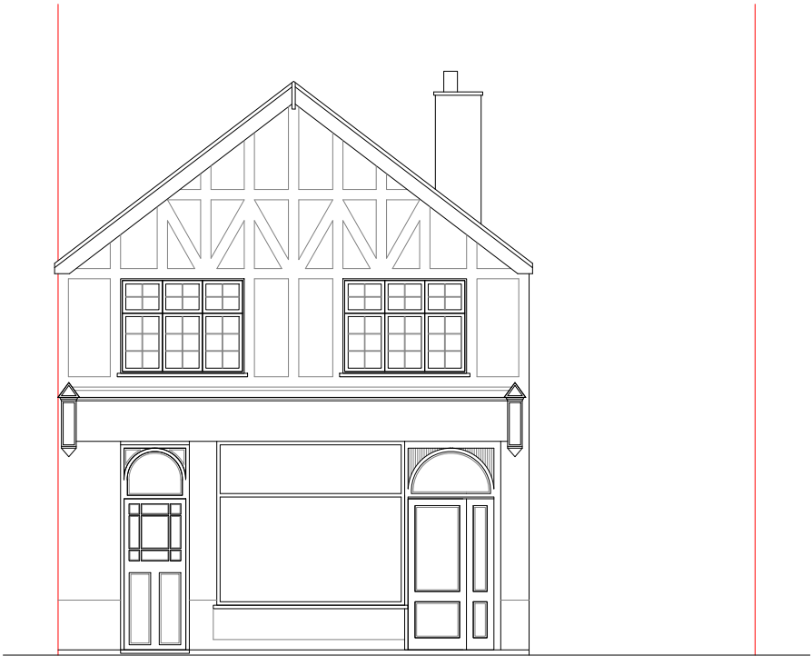
Proposed Front Elevation Scale 1:100
