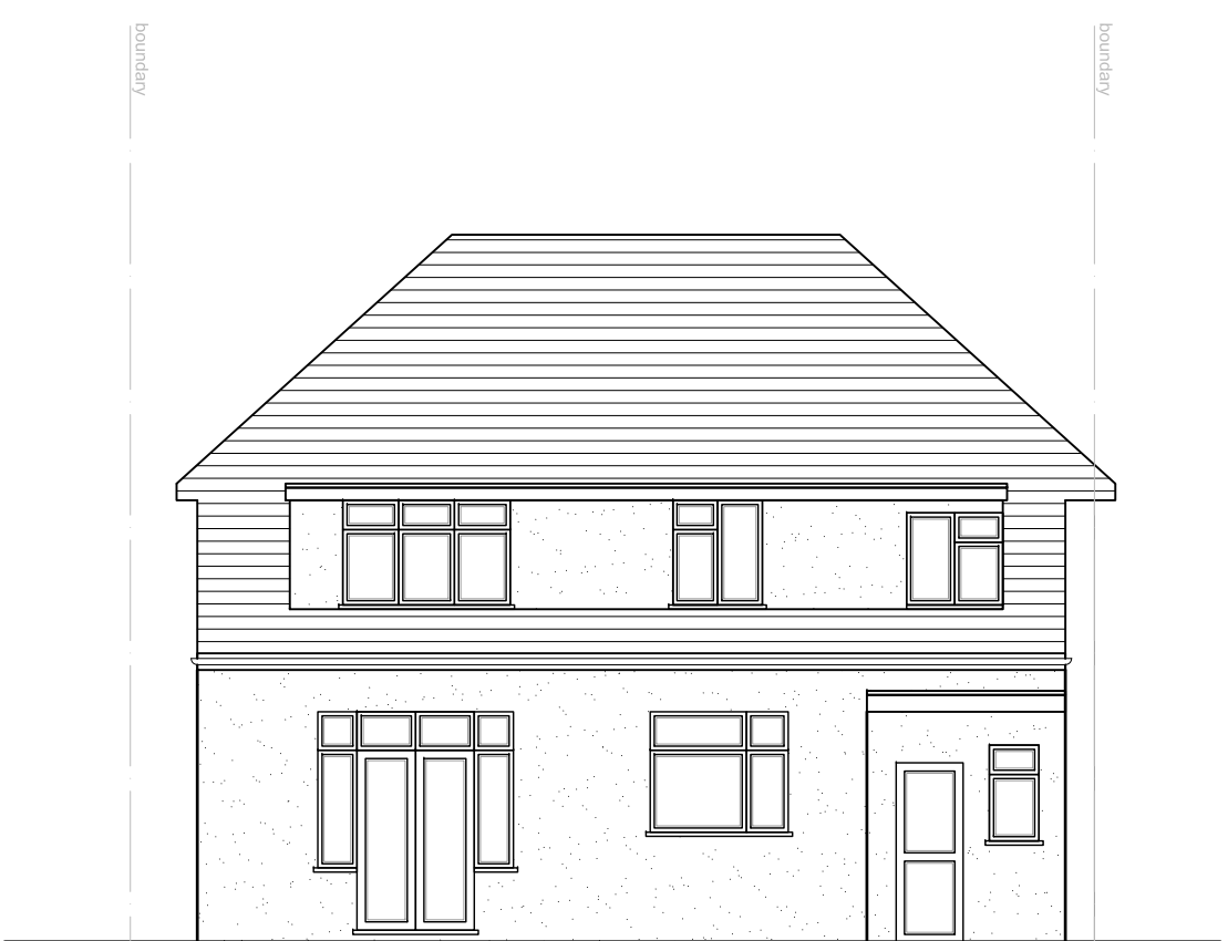
EXISTING REAR ELEVATION
