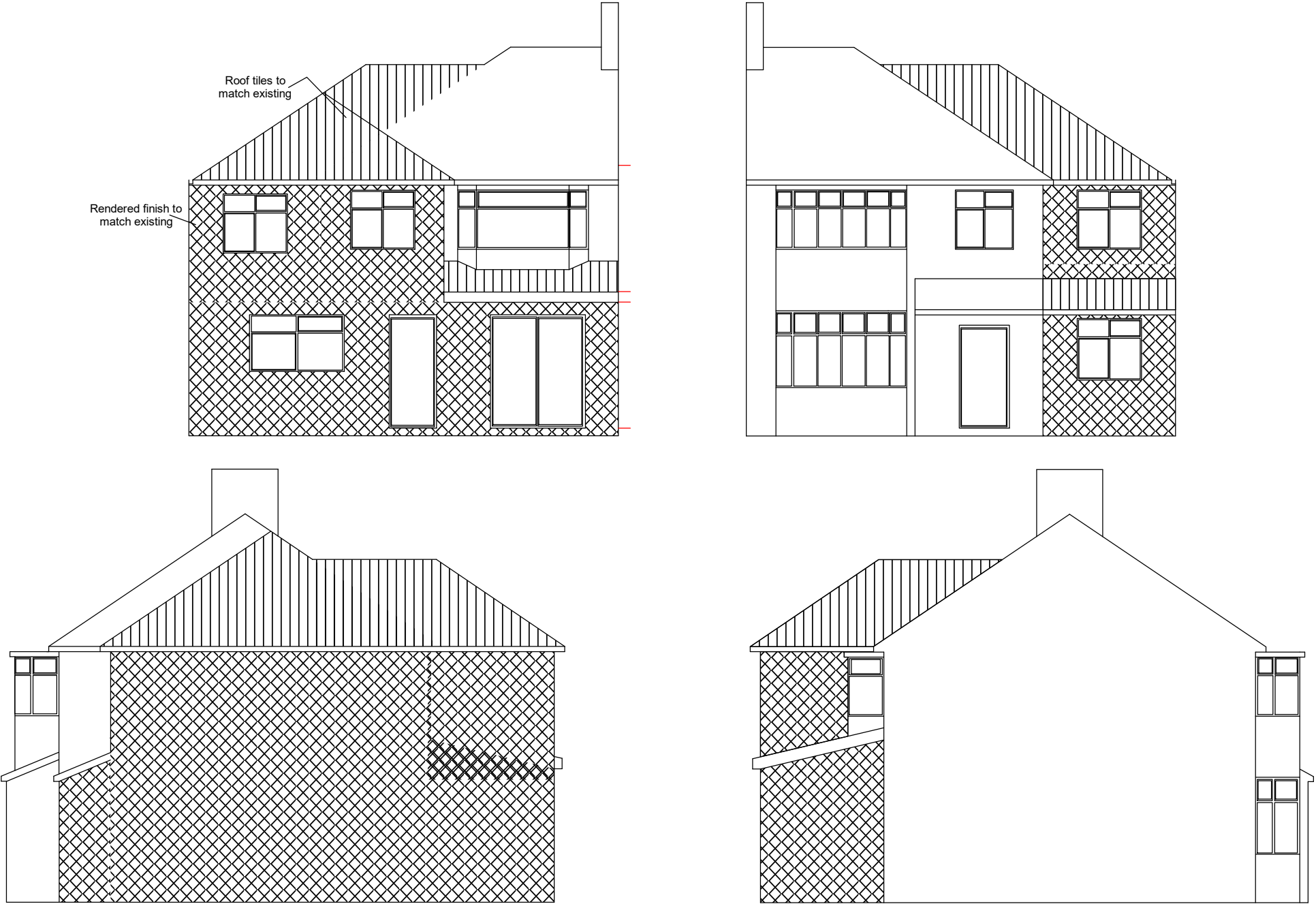
PROPOSED REAR / FRONT & SIDE ELEVATIONS Scale 1:100
