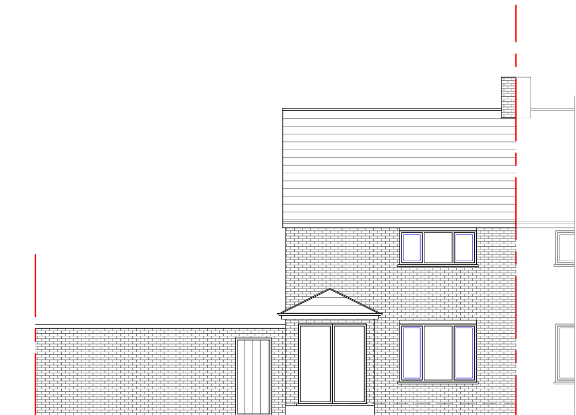
NO.14 NO.12 EXISTING FRONT ELEVATION
