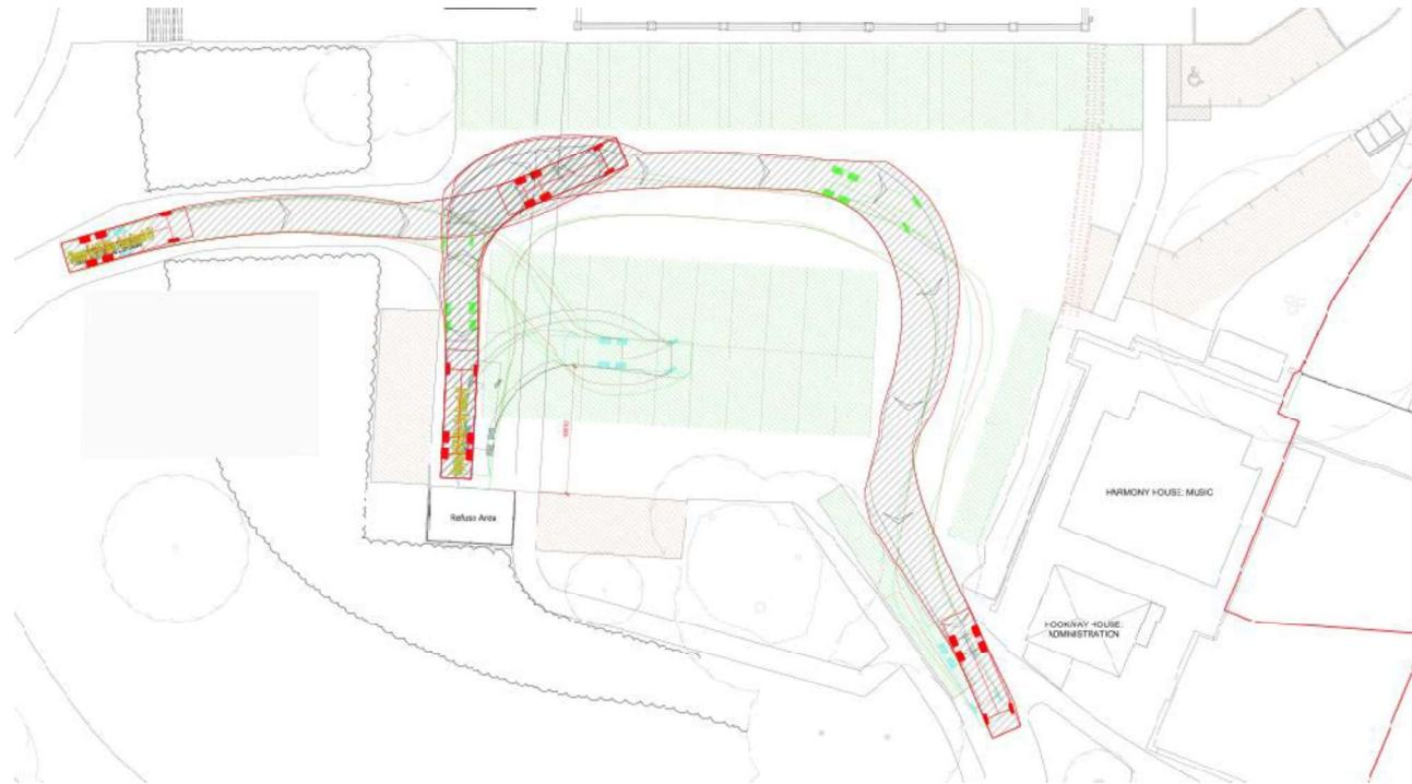
*Snip showing route of rear-loading refuse vehicle (Green bays are coach drop-off/ pick-up bays – in the event these are full, a large refuse vehicle can manoeuvre through the site)*
