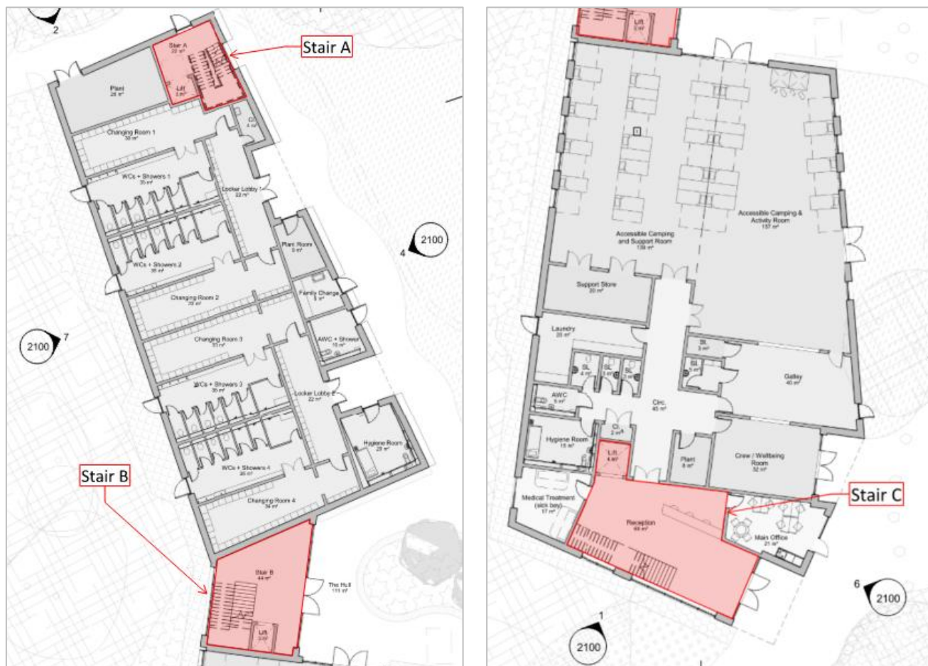
Figure 9 – Operations Zone Protected Stair Cores
