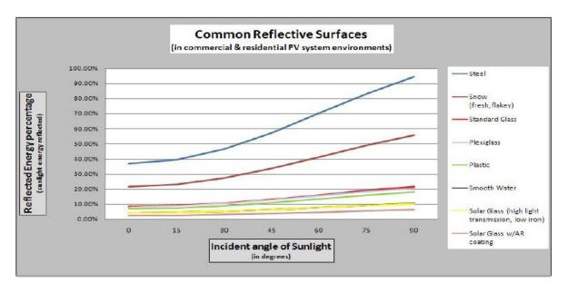
It should be noted that the reflected energy percentage of Solar Glass is far below that of a standard glass and more on the level of smooth water. Also, below are the ratios of the common reflective surfaces:
