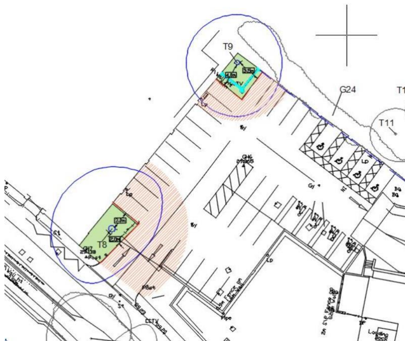
Image 1: areas of existing hard surfacing to be retained until broken and removed under arboricultural supervision.
