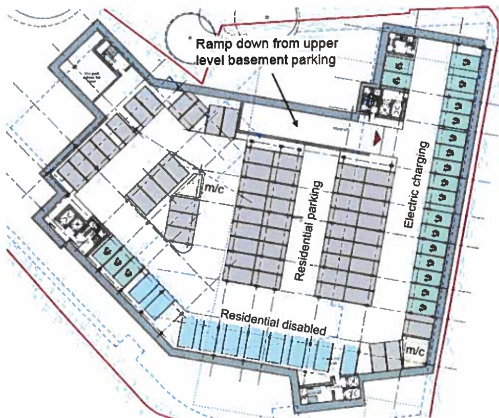
Figure 2.3 Lower Level Basement Parking Provision (Level 2)
