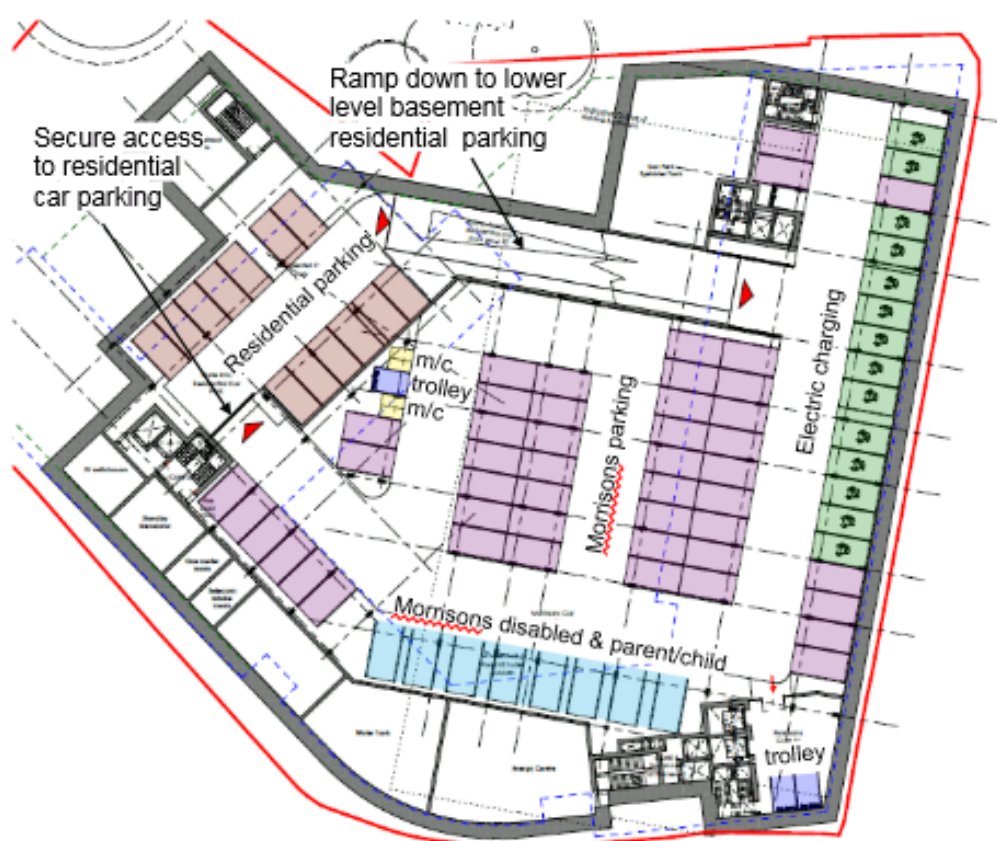
Figure 3.1 Upper Level Basement Parking Provision (Level 1)
