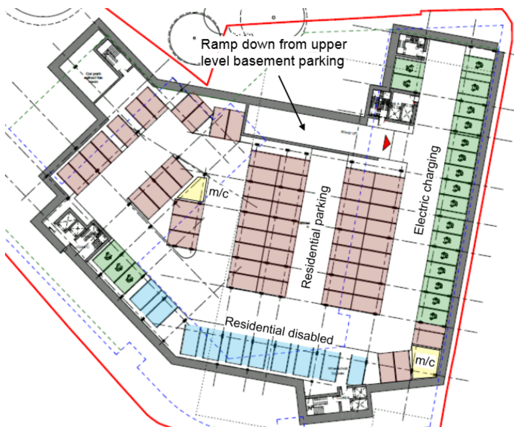
Figure 3.2 Lower Level Basement Parking Provision (Level 2)
