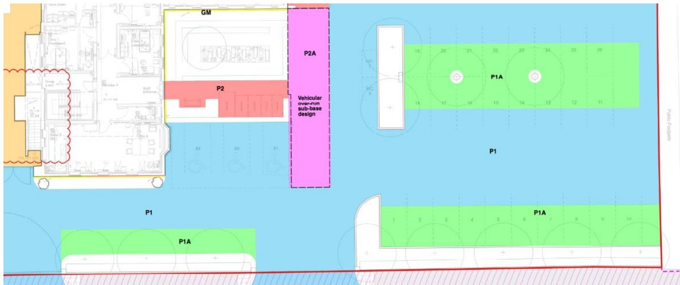
The role of the Permeable Bitumen Macadam Surface over the tree pits is to allow soil aeration and permeability of water for irrigation of the trees.
