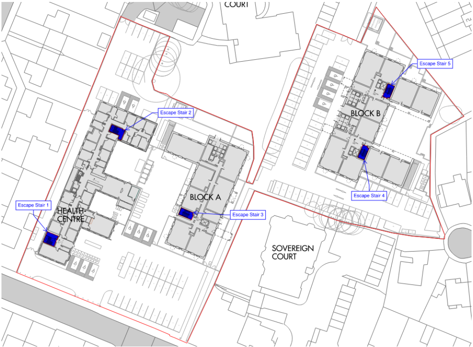
Figure 5: Illustration showing all escape stairs in blocks A, B and healthcare.
