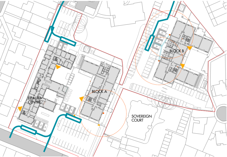
Figure 7: Illustration showing the fire service vehicle access points and points of entry (A&M planning drawing)
