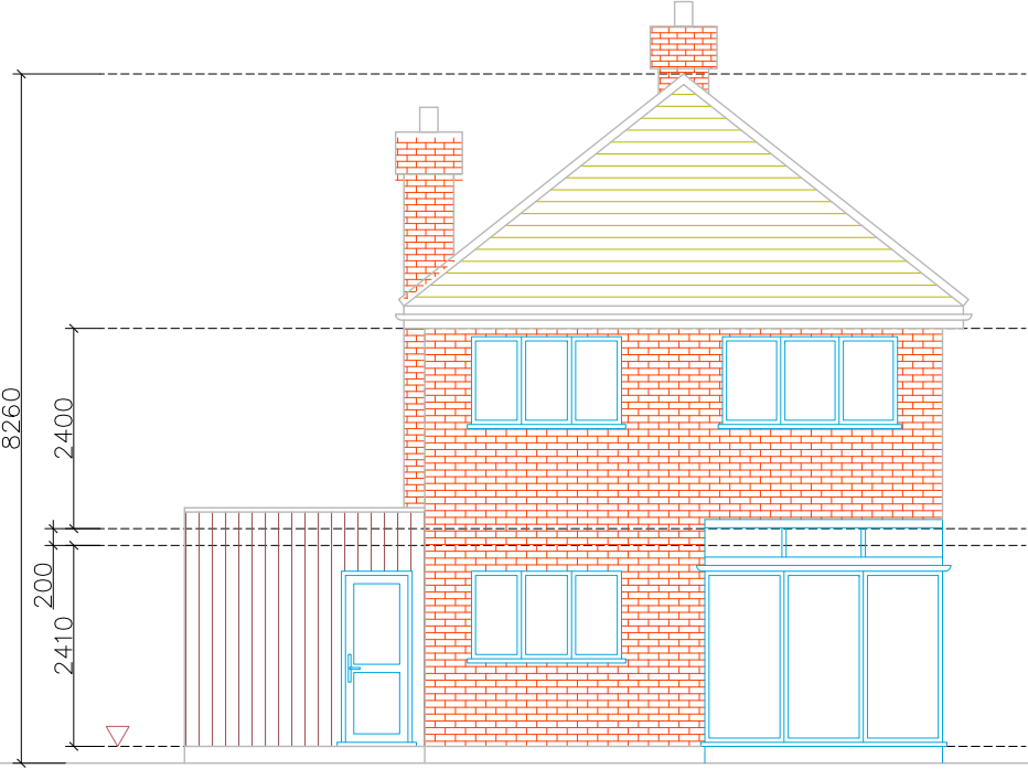
EXISTING REAR ELEVATION
