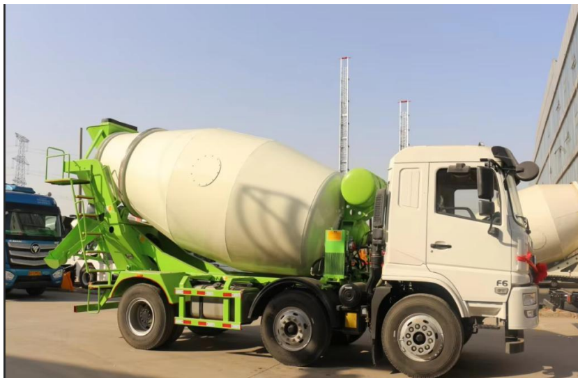
Small concrete wagons
