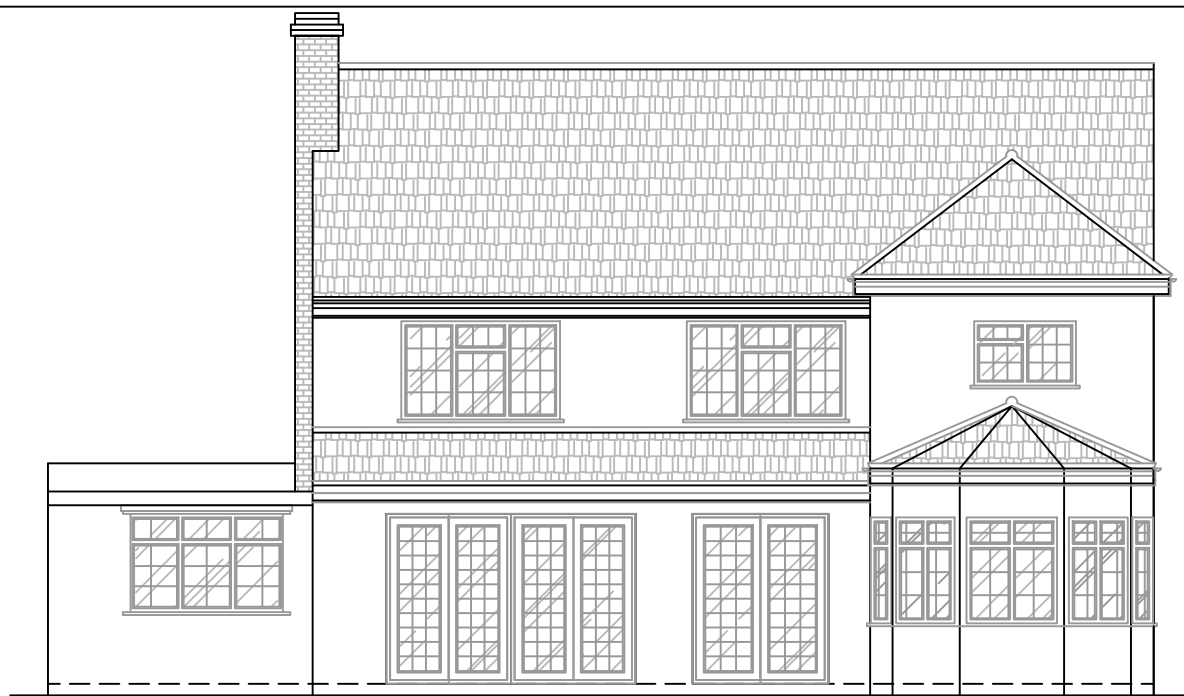
EXISTING REAR ELEVATION
