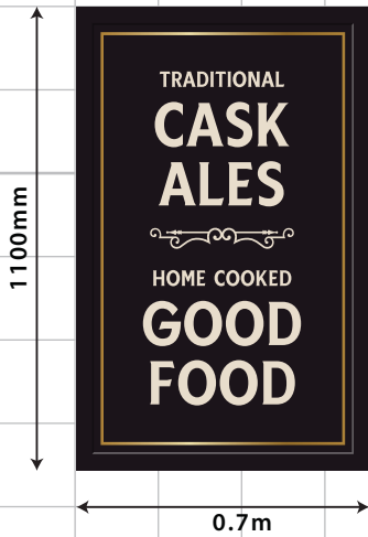
F ONE X NEW AMENITY BOARD SIZE. 0.7m x 1100mm. H.A.G. 0.9m.
