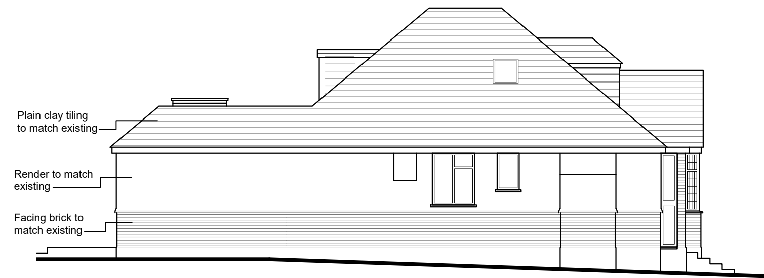
PROPOSED SIDE (NORTH EAST) ELEVATION
