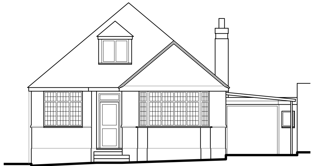
EXISTING FRONT (NORTH WEST) ELEVATION
