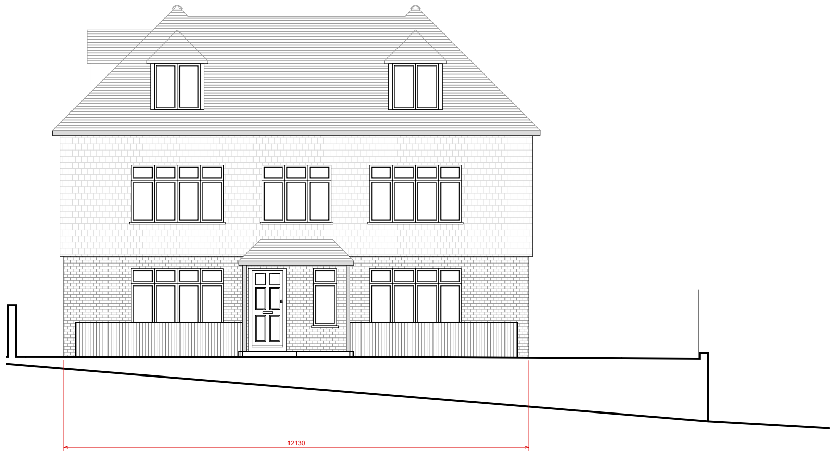
Proposed Front Elevation Scale 1:100
