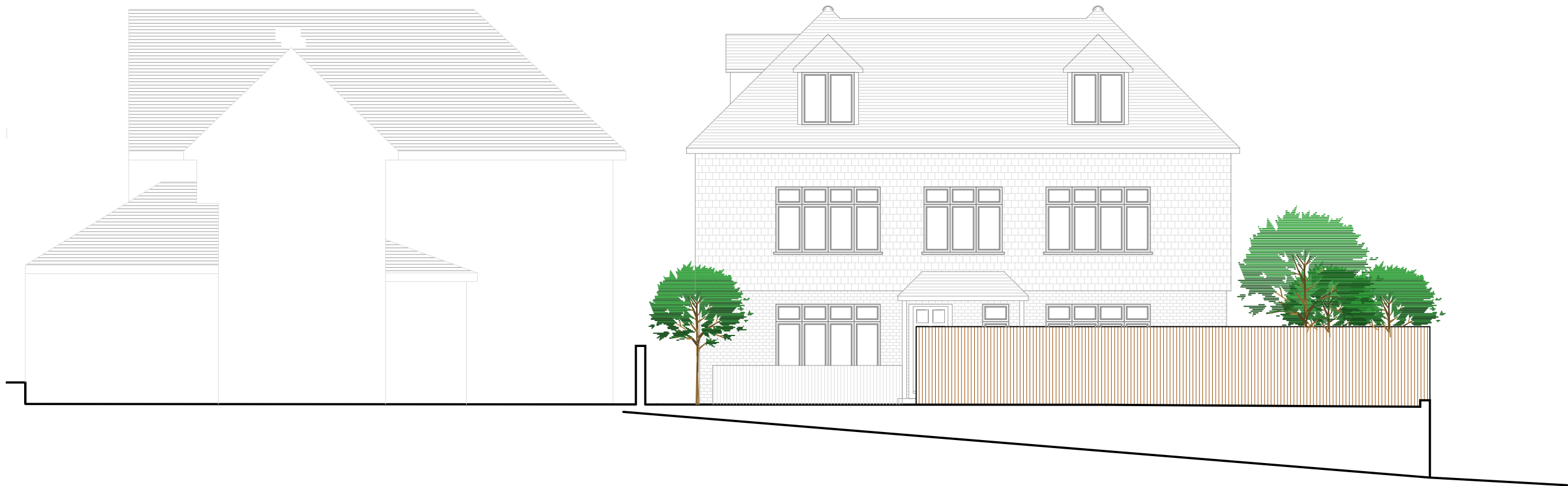
Proposed Front Elevation Showing Boundary Treatment Scale 1:100
