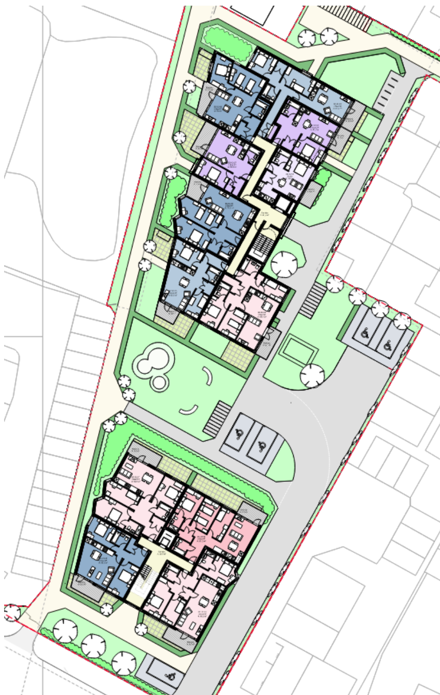
Figure 4. Block 1 & Block 2 Second Floor Layout
