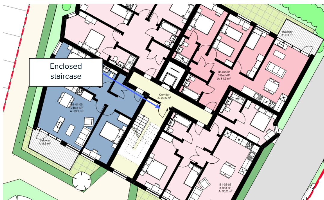
Figure 6. Block 1 common corridor design
