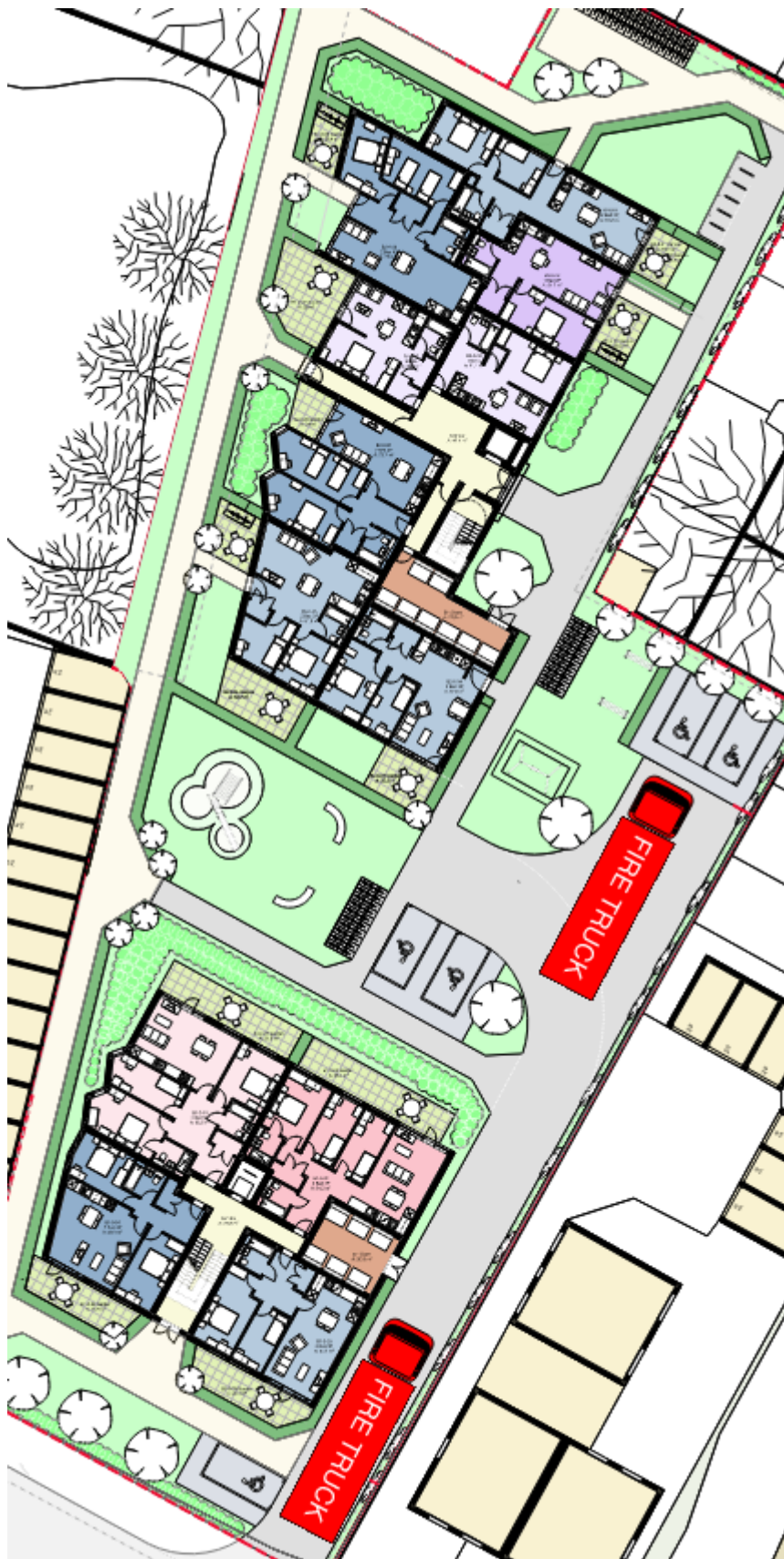
Figure 12. Fire Service Access
