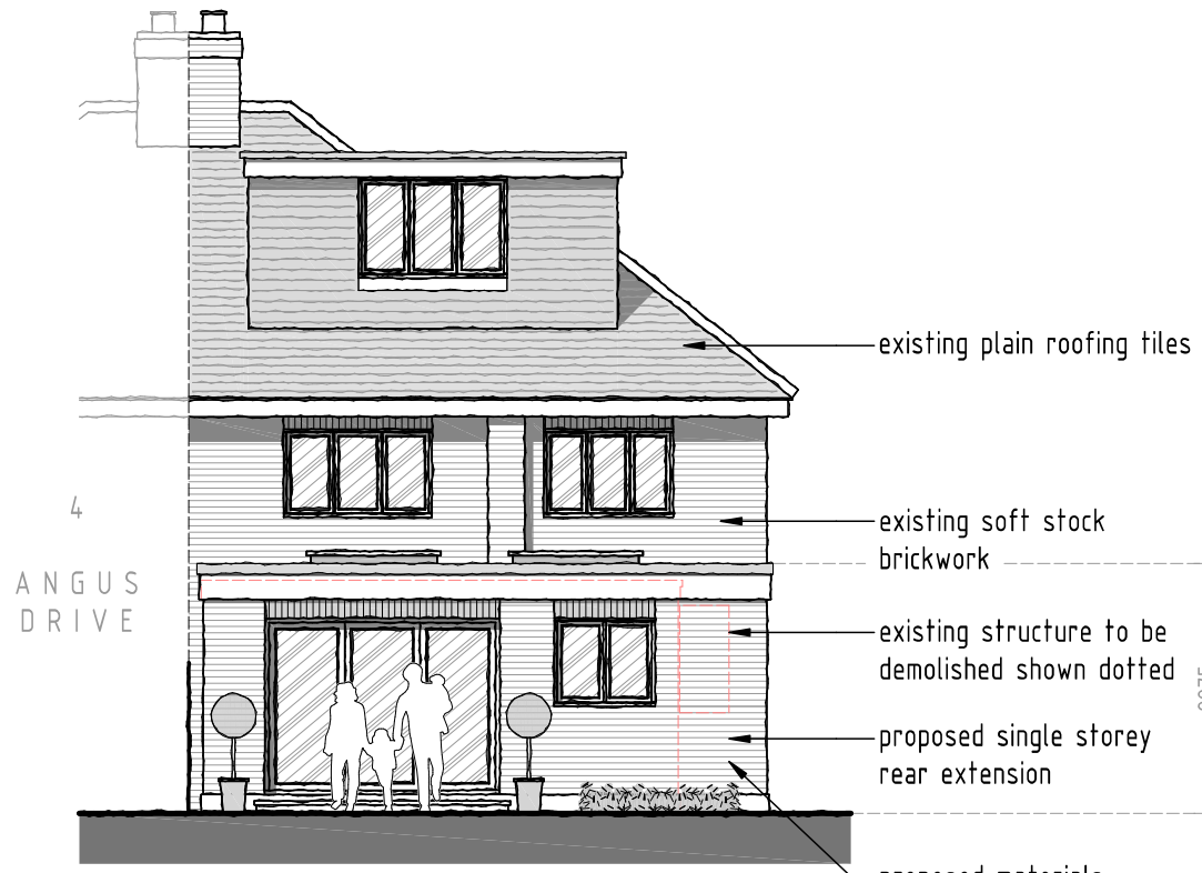
PROPOSED REAR ELEVATION SCALE 1:100
