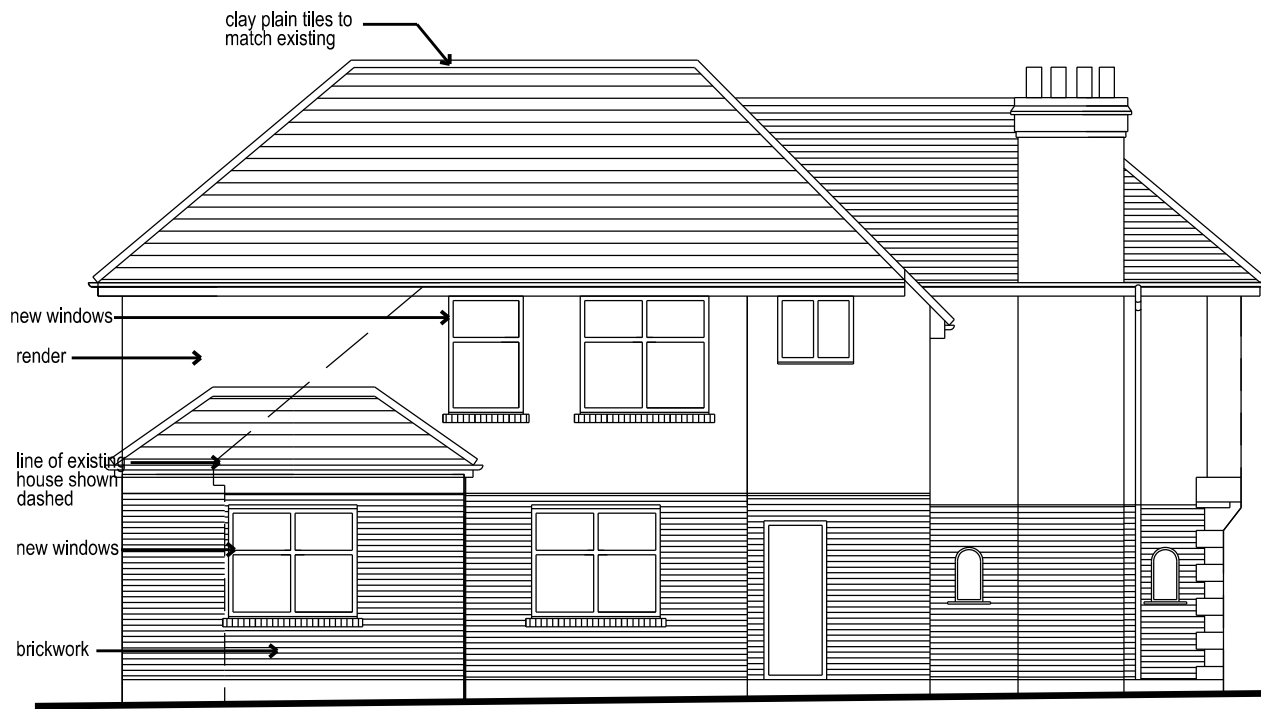
SOUTH WEST ELEVATION
