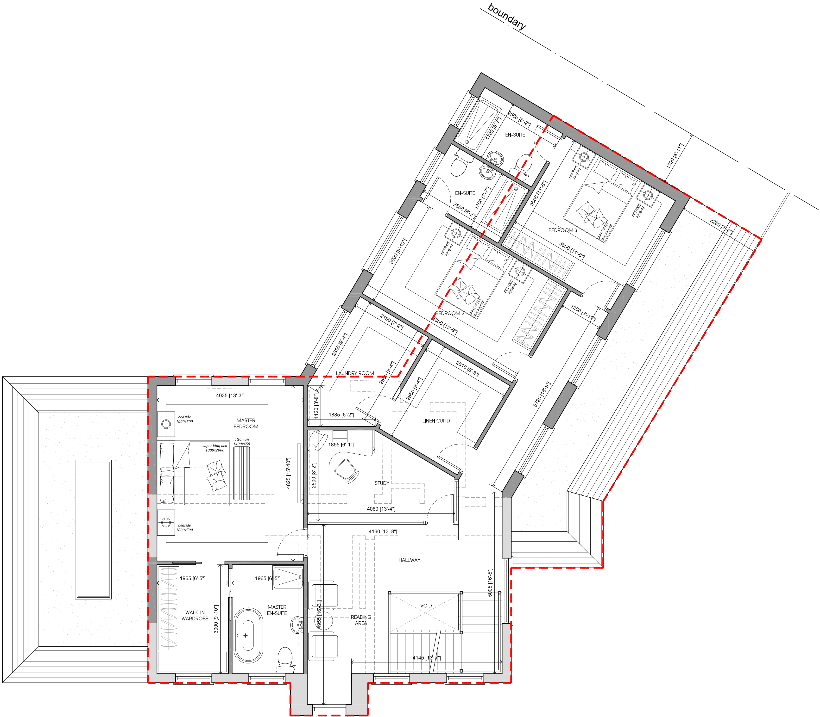
PROPOSED FIRST FLOOR PLAN FLOOR AREA : 126 m 2 / 1356 ft 2 TOTAL FLOOR AREA : 378 m 2 / 4069 ft 2
