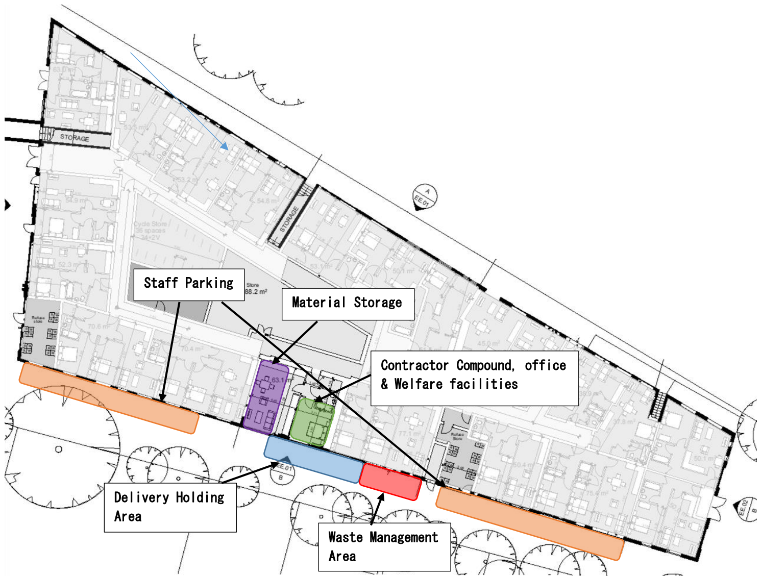
Figure 2: Proposed Site Layout during construction, showing where the staff parking, on-site welfare facilities, material storage and waste management areas will be located
