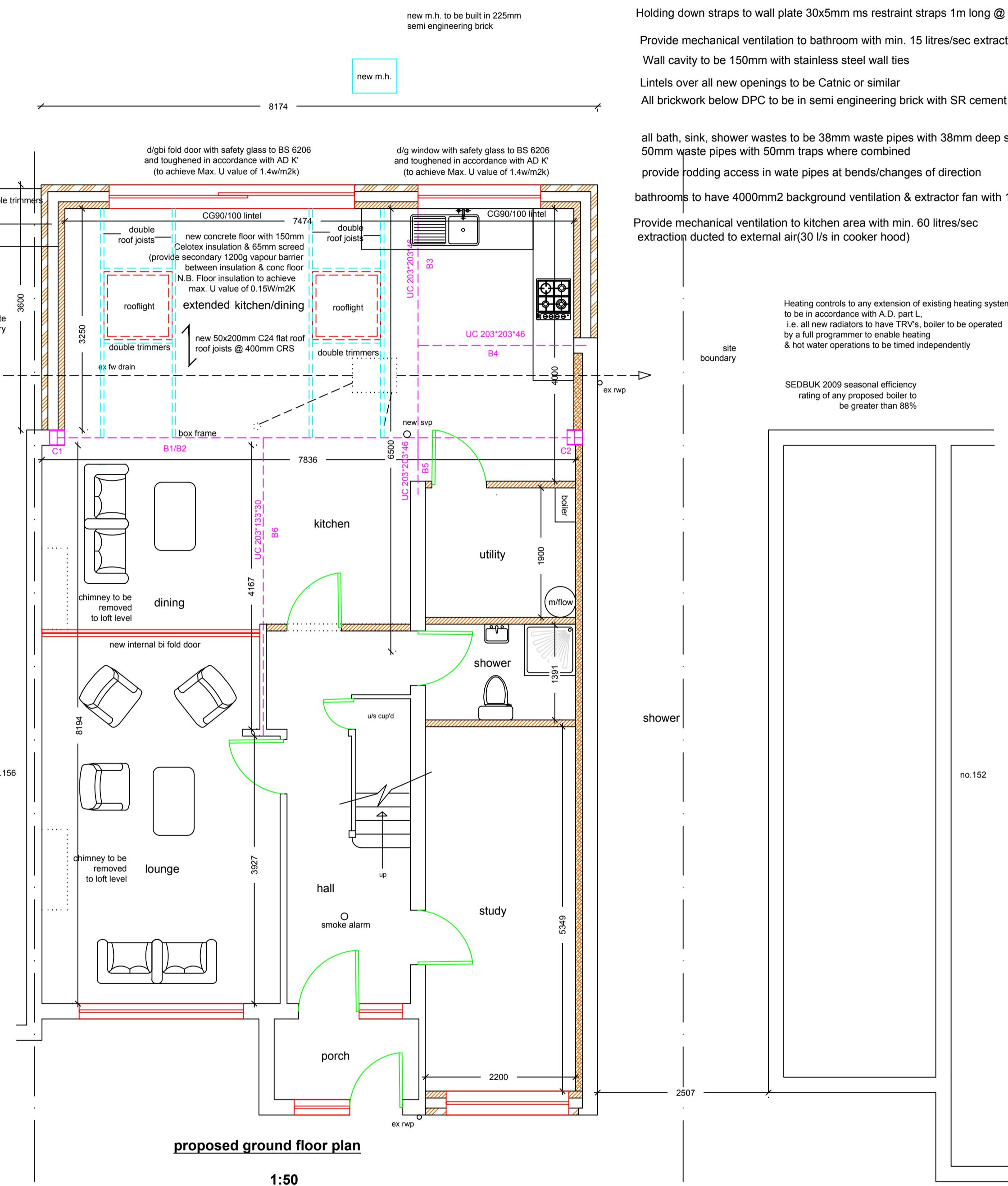
1. Proposed foundations min depth 1.0m & 500mm wide or 600mm wide for eccentrically loaded foundations
