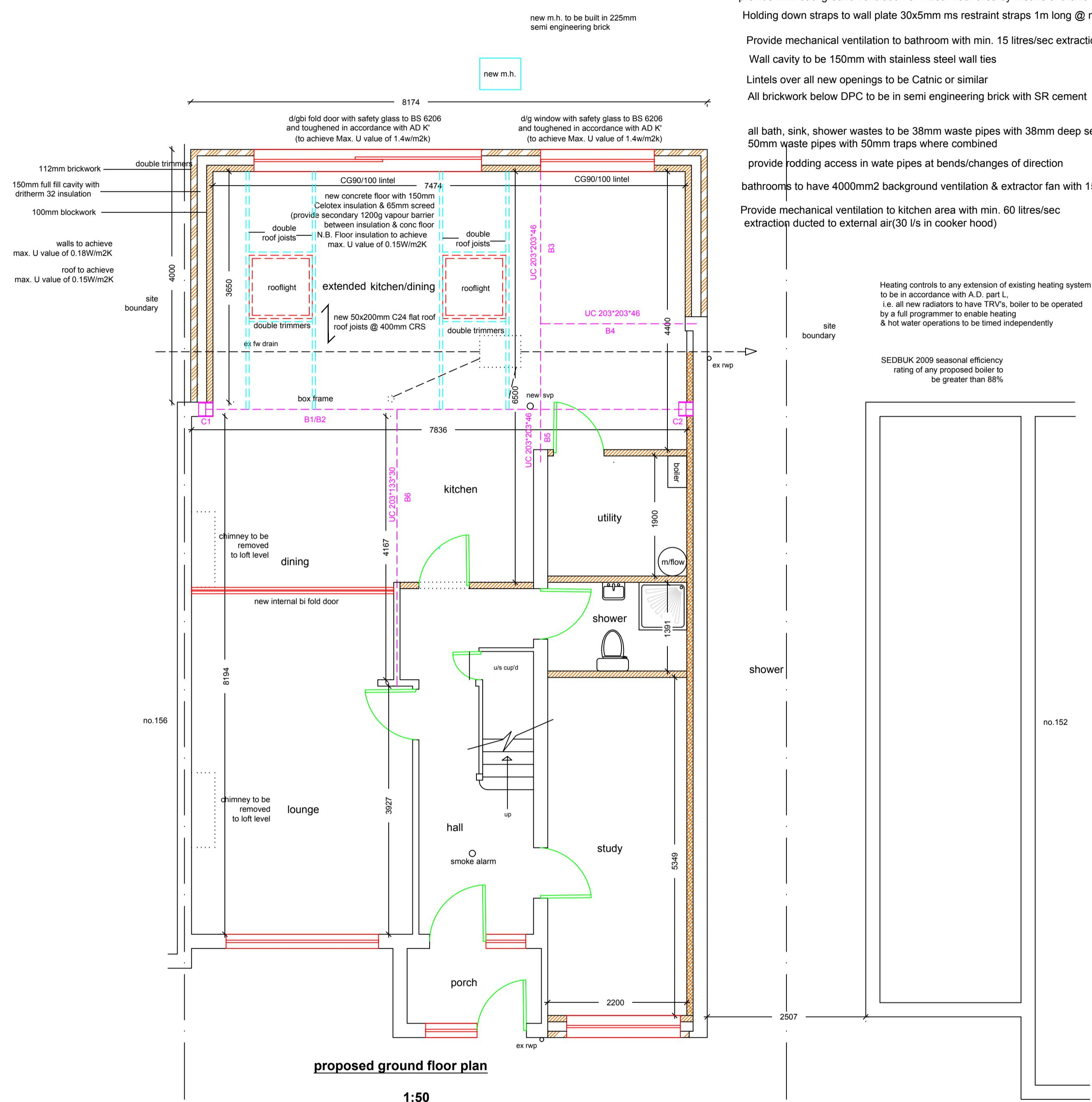
1. Proposed foundations min depth 1.0m & 500mm wide or 600mm wide for eccentrically loaded foundations
