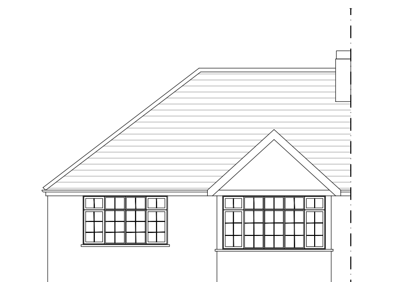
PRE-EXISTING FRONT ELEVATION
